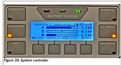
using 1.5 KW (bottom bar. The right half of the split center bar shows the system selling 0.1 KW (100W) to the utility. This small amount is barely visible on the bar graph.
