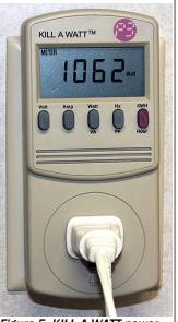
Figure 5: KILL A WATT power monitor in use
