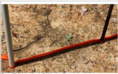
Figure 13: Using stakes to find true north
