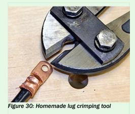
We bought a 24" bolt cutter for \$13 at Wal-Mart, disassembled it, and ground semi-circles in the jaws. It works well.
